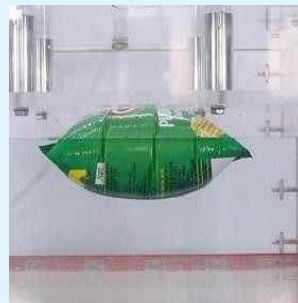
Faulty Seal - See the Air Bubbles!
